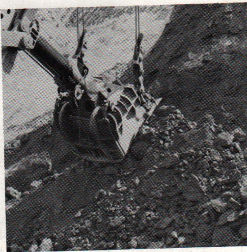
The side of the pit has been broken up by blasting, and the Bucyrus Erie shovel digs in.
