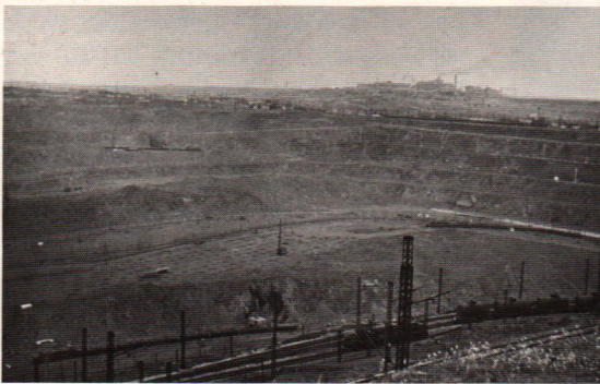
Open-pit taconite operations on the Krivoy Rog are similar to those on Minnesota's Mesabi Range. Note concentrating plant in the background in left photo. (Unfortunately, these color-slide snapshots lose considerable contrast when printed in black and white.)
