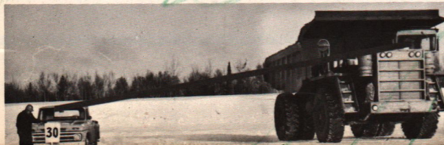
FOR A 65-TON DART, THE DANGER DISTANCE INCREASES TO 30 FEET.
