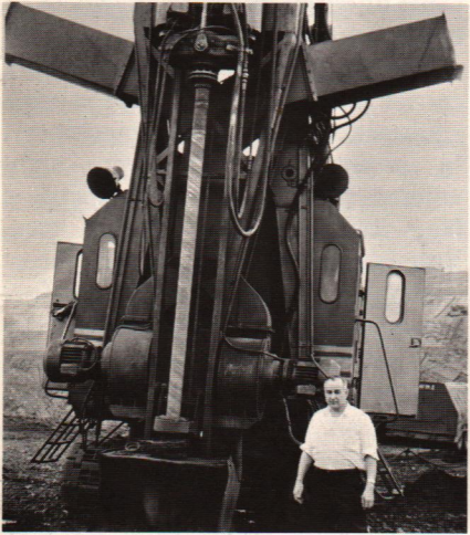
No, this picture was not taken at Erie Mining Company! PM's Bob Bell poses with a Russian jet piercing drill, used to bore blast holes in the Krivoy Rog taconite.
