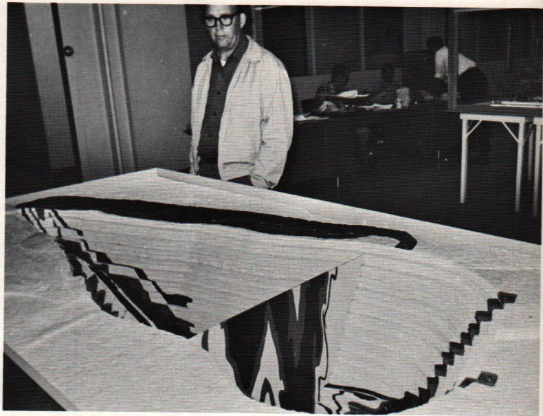
Visitors and new employees get their first view of the mine and plant from scale models. The model of the plant, built by the prime construction contractor, proved to be such a valuable training aid that a similar model of the mine pit was constructed of styrofoam, with removable sections to show the progression of mining over the expected economic life of the deposits.
