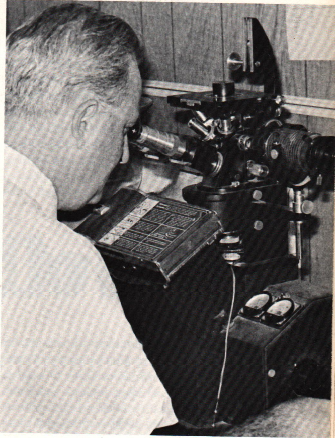
Microscopic examination of zirconia ceramics enables close control of their physical properties. Shown operating the camera-equipped microscope is A. G. King, Zircoa's technical director.
